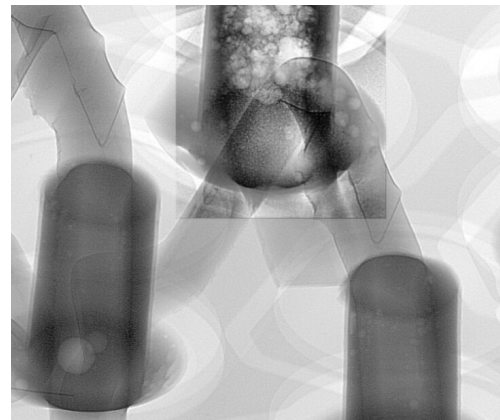
THT with voiding
